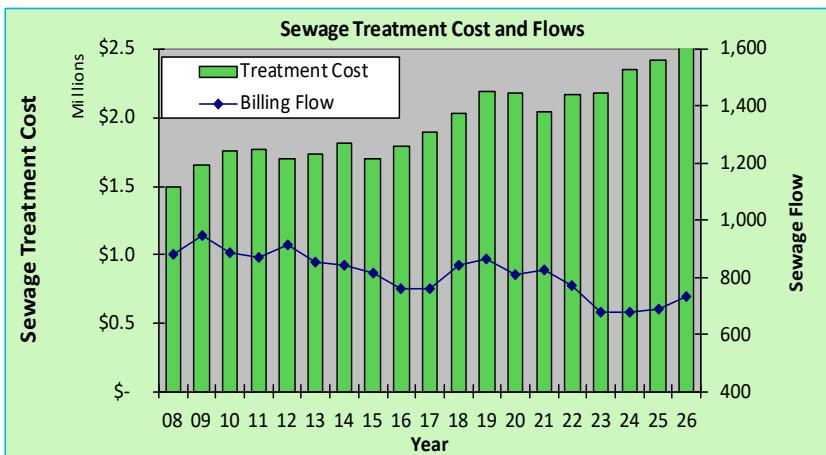
Sewage flows can also be impacted by groundwater infiltration and storm water inflow, particularly during periods of heavy downpours. Cracks in sewer lines, openings in manholes, and illegal connections of roof drains and/or sump pumps to the sewer system allow water to flow directly into sewer pipes, which in turn drives up sewer flows and sewage treatment costs.
