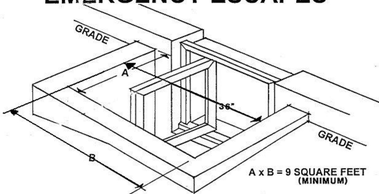
The clear horizontal dimensions shall allow the window to be fully opened and provide a minimum accessible net clear opening of 9 square feet, with a minimum dimension of 36 inches.
