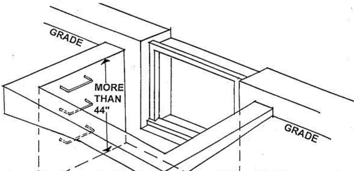
Window wells with a vertical depth of more than 44 inches shall be equipped with an approved permanently affixed ladder or stairs that are accessible with the window in the fully open position. The ladder or stairs shall not encroach into the required dimensions of the window well by more than 6 inches.
